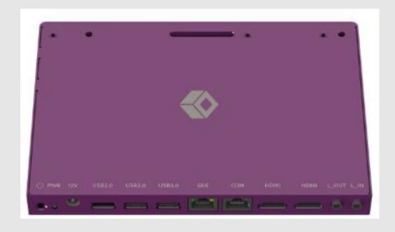
CPU: Intel® Atom; Quad-Core, 1.91 GHz
